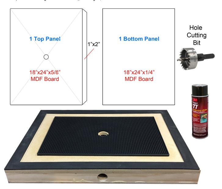
Cut the 1"x2" board into (2) 24" and (2) 16.5" sections. Glue & clamp first 1"x2"x24" to top panel. Then glue & clamp The two 1"x2"x16.5" to top panel. Before adding the last 1"x2"x24" section dill the hose hole then Glue & clamp to complete box frame.
