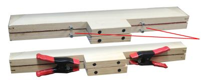
Side screws for Clamps. Without these EVA foam will pull out of frame.
