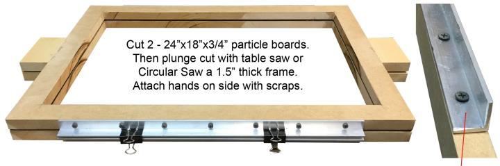
Cut the 3/4" aluminum angle into four 18" sections. Then drill 7 holes evenly spaced as shown.
